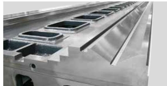
**COMPOSITAL** a new solution composed by resine-granite mixture filled on welded-steel casing that permit to:
